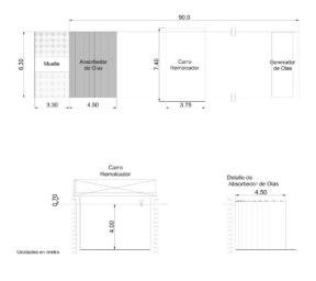
An IRR of 9% and a NPV of \$ 282,372.25 were obtained, recovering the investment in 9 years, for a towing tank with the following dimensions 90x6,3x4 m, that will allow tests with models at a scale of 2.5 m at a maximum speed of 5 m / s (1.00 Fn), in calm waters or in waves, replicating the region's sea to a level 5 sea state.
